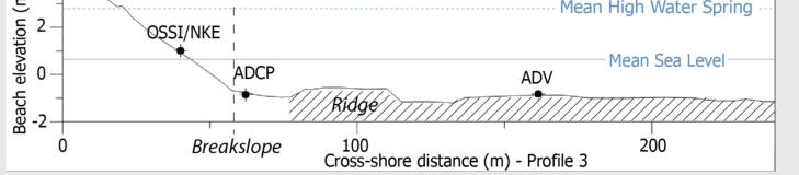
Cross-shore topographic centrale profile ; location of instruments on reflective and dissipative parts
