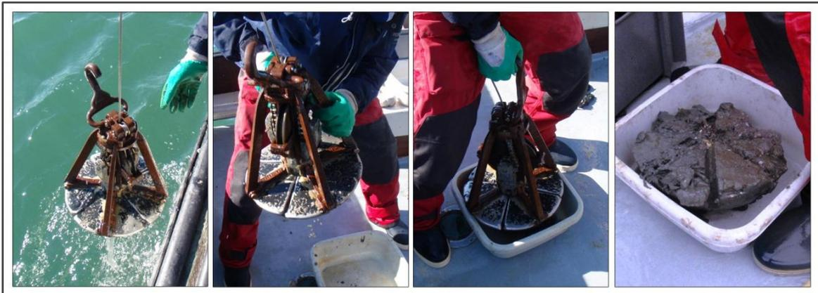
**Figure 2-21.** Processes obtaining surficial sediments by Orange Peel grab.
