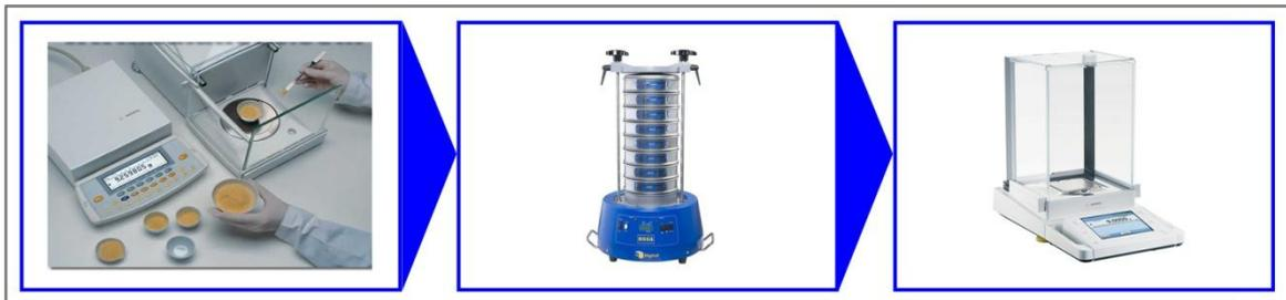
**Figure 2-30.** Dry sieving procedures for coarse fraction sediments.
