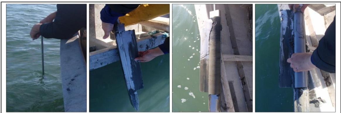
**Figure 2-24.** Processes obtaining the core sediment by D-section corer.
