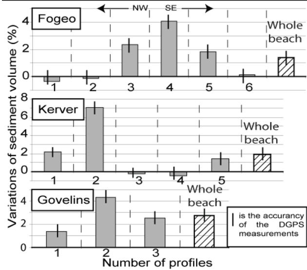
Figure 6: Variations of sediment volume calculated from the profiles of the Fogo, Kerver and Govelins beaches surveyed in February and March 2010.
